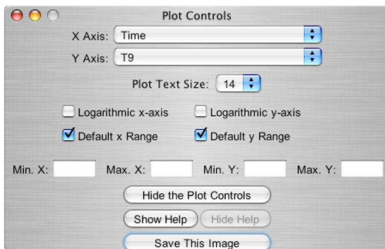
FIGURE 6: This is the control panel for the simple 2-D image plotter. Users can choose to view the various data on either axis, and they have control over log scales, axis range, and the text size. They can also view help information from this panel as well as save the image once they are satisfied with the way it looks in the main browser window.
